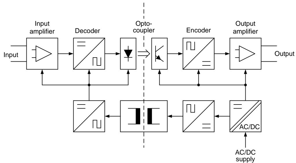
TDG-210DG requires auxiliary voltage and is fed through a transformer or a 24/48/110/220 V DC inverter. The secondary voltage is rectified and fed to the encoder and output amplifier shown to the right of the galvanic interface. The input amplifier and the decoder are fed through a DC/DC inverter. The input signal is amplified and is, through optocouplers, transmitted to the output amplifier.
