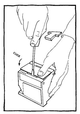
Press with a screwdriver as indicated by the arrow and press the front panel down with your thumb, simultaneously. It is recommended that one side of the front panel snaps into place before the other.
