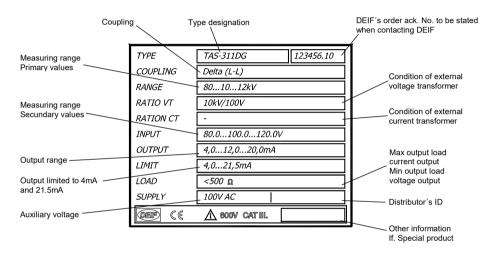
The un-configured transducer is provided with a label with the following data:
