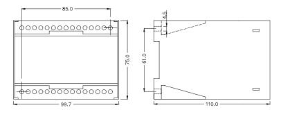
The RMV-142D is designed for panel mounting, being mounted on a 35 mm DIN rail, or by means of two 4-mm screws.
