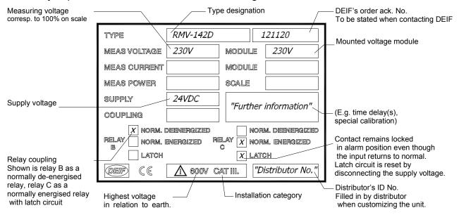
Note: The relay is provided with a 200 ms power-up relay, ensuring correct function of the relay on connection of the auxiliary voltage. Normally energised contacts ("NE") are not activated (contact does not open/close) until 200 ms after connection of the auxiliary voltage. Likewise, the relay is provided with a 200 ms power-down circuit, ensuring supervision and maintenance of any set point exceeding for 200 ms after disconnection of the auxiliary voltage.
