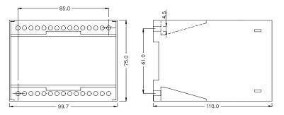
The RMV-122D is designed for panel mounting, being mounted on a 35 mm DIN rail, or by means of two 4-mm screws.
