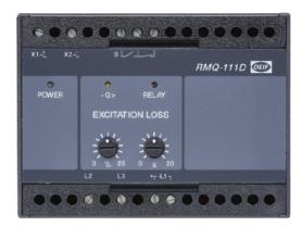
This Uni-line relay protects generators running in parallel with other generators from running as an induction generator due to under-excitation – particularly in cases where applying an under-voltage relay for protection is insufficient.
