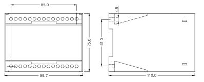
The RMP-112D is designed for panel mounting, being mounted on a 35 mm DIN rail, or by means of two 4-mm screws.
