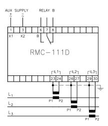
A 2A fuse may protect the auxiliary supply connection.
