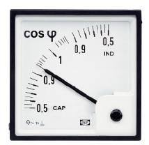
The PFQ power factor meter measures cos phi with a moving coil movement and an electronic transducer. The transducer measures the phase angle between an AC voltage and the corresponding AC current, converting the signal into a proportional DC current which is then fed to the moving coil instrument.
