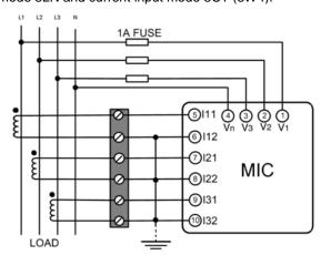
Principle diagram for 3LN, 3CT Connection (3W4)
