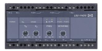
DEIF's Uni-line Load Sharing Unit, the LSU-114DG, provides load sharing with automatic start/stop outputs between generators and interfaces to a governor through an electronic potentiometer (EPQ96-2 or EPN-110DN).
