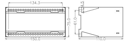
The LSU-112DG is designed for panel mounting, being mounted on a 35 mm DIN rail, or by means of two 4-mm screws.
