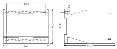
The LMR-122D is designed for panel mounting, being mounted on a 35 mm DIN rail, or by means of two 4-mm screws.
