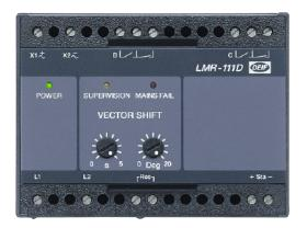
The Loss of Mains Relay Uni-line LMR-111D is for protection of the generator against damage resulting from a non-synchronised reconnection to the grid after a temporary mains failure.
