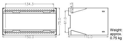
The design of the paralleling relay makes it possible to mount it close to other *uni-line* units. However make sure there are min. 50 mm between the top and the bottom of this relay and other relays/units. The DIN rail must always be placed horizontally when several relays are mounted on the same rail.
