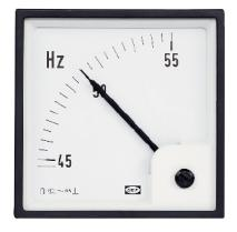
With high immunity to 3<sup>rd</sup> harmonics, DEIF Pointer frequency meter is suitable for all applications. The moving coil instrument features integrated electronics for converting frequency into analogue readings with accurate and linear readouts on an exchangeable scale
