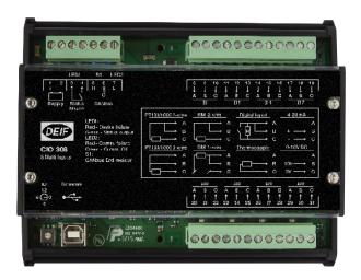
The CIO 308 is an external I/O module for DEIF's Multi-line series for those requiring a number of inputs exceeding the capacity of a range of DEIF genset controllers.
