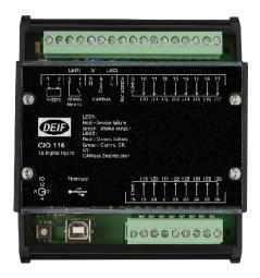
The CIO 116 is an external I/O module for DEIF's Multiline series for those requiring a number of digital inputs exceeding the capacity of a range of DEIF genset controllers.
