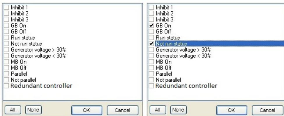
Inhibit of the alarm is active, as long as one of the selected inhibit functions is active.
