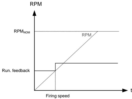
The diagram illustrates how the digital running feedback is activated when the engine has reached its firing speed.
