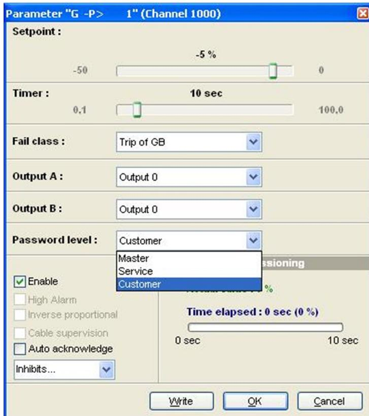
The password level can also be changed from the parameter view in the column "Level".
