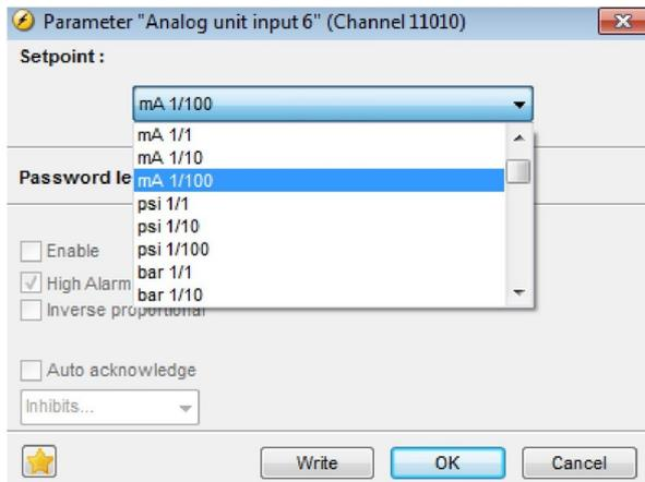
6. It is necessary to read the parameters from the device to the computer after changing the scale (1/1, 1/10 or 1/100) settings. This is in order to refresh the parameter list so the alarm settings present the correct value.
