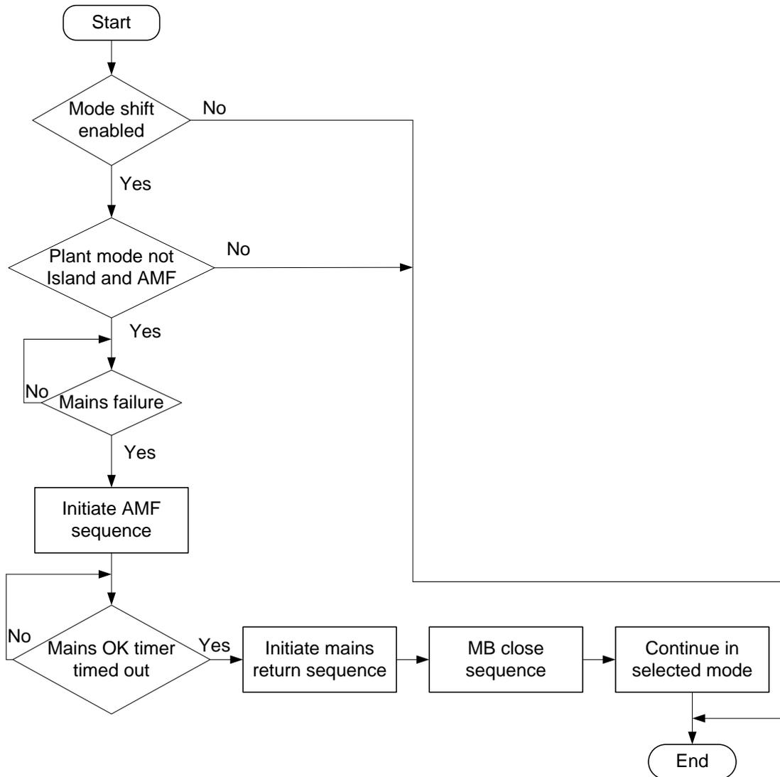
**i** To enable mode shift, a digital input has to be set up.
