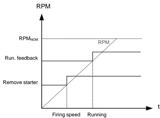
The diagram illustrates how the remove starter input is activated when the engine has reached its firing speed. At the running speed, the digital running feedback is activated.
