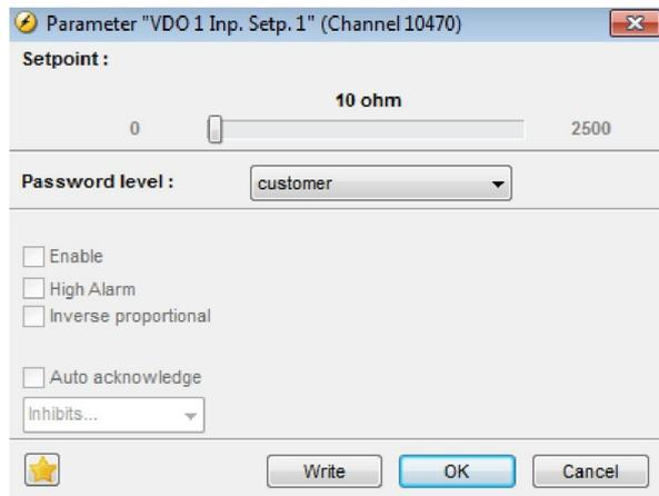
Adjust the resistance of the RMI sensor at the specific measuring value. In the example above the adjustment is 10  $\Omega$  at 0.0 bar.
