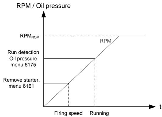
**i** The remove starter function can use the MPU or a digital input.
