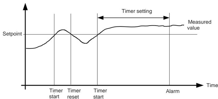
When the timer runs out, the output is activated. The total delay will be the delay setting + the reaction time.
