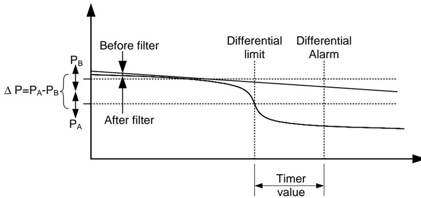
Three different differential measurements between two analogue input values can be configured.
