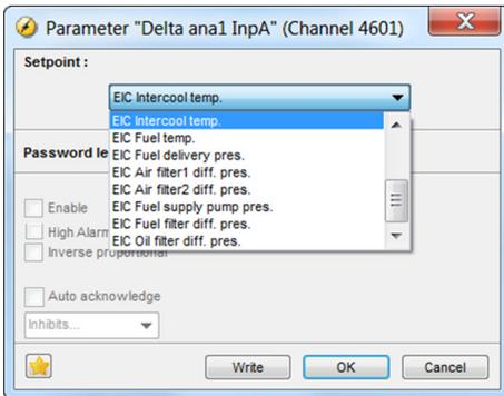
The relevant alarm setpoint is chosen in parameters 4610-4660. Each alarm can be configured in two alarm levels for each differential measurement between analog input A and input B. Below figure shows the two parameters to configure alarm level 1 and 2, for differential measurement 1.
