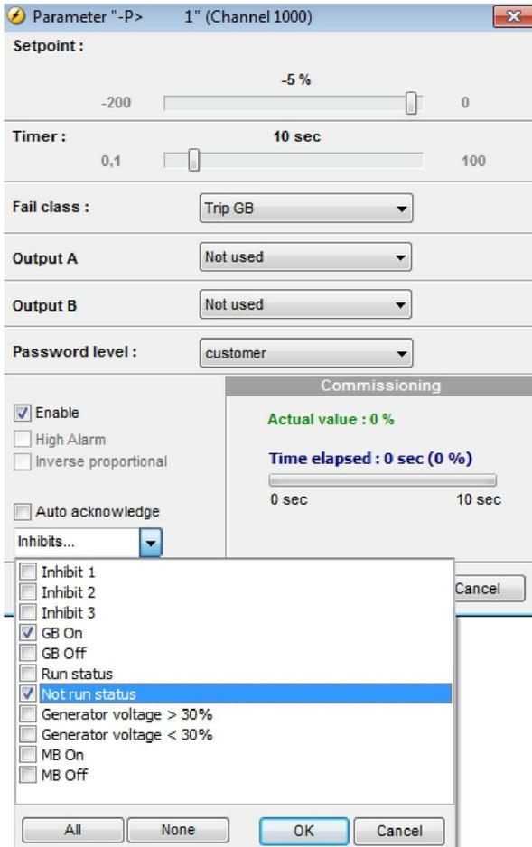
In this example, inhibit is set to *Not run status* and *GB ON*. Here, the alarm will only be active when the generator is running and disabled again when the GB is closed.
