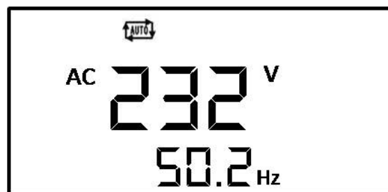
Example: Genset AC voltage and frequency (Hz)
