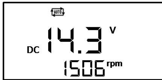
Example: Battery DC voltage and genset running speed (RPM)
