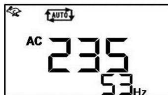
Example of over-speed alarm
