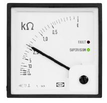
The ADL-111Q96 is used to supervise the insulation resistance between an isolated voltage distribution network and an earth/safety cable. The insulation monitor is applicable with DC networks for voltages of 24, 110 or 220 V DC. The ADL-111Q96 has a relay output with adjustable set point, and it can be configured to either NE (normally energised) or ND (normally de-energised).
