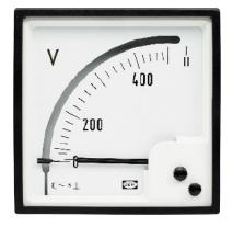
2EQ double voltmeter has two mutually independent moving iron systems with a joint scale. The point of rotation for both systems is at the lower right corner.
